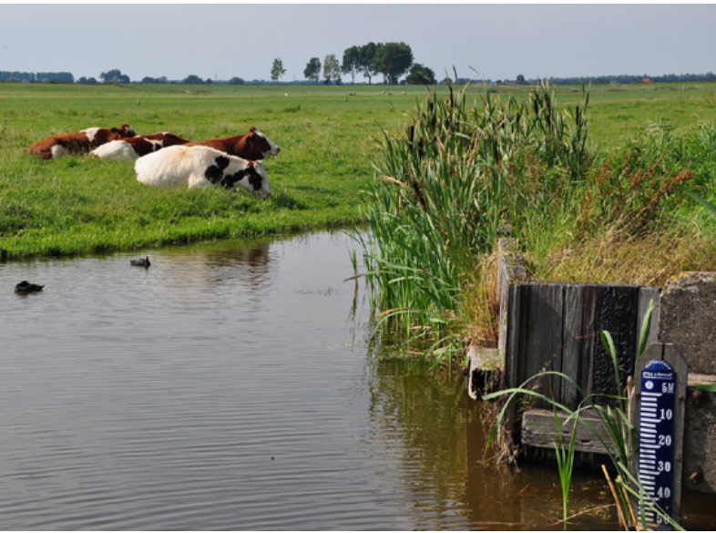
A scale measures water levels in a polder, Zoetermeer, Netherlands. (Vincent van Zeijst / Wikimedia Commons )
